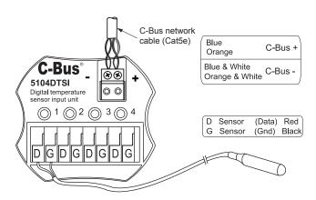
The input unit can support the connection of 1 to 4 sensors. Only one sensor can be connected per input channel. Unused channels are allowed.
