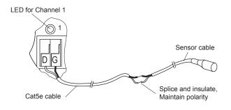
The extended sensor cable for an input channel must not exceed 25m. Use twisted pair cable that is not pink (colour of the C-Bus cable).
