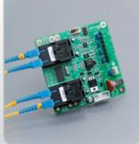
**Note:** Single Mode Fibre Modem (995087) is supplied in the same plastic enclosure as the Multimode Fibre Modem (995081). There is also provision to mount Fibre Modem PCBs in the Low Profile Enclosures along with Control Module and Expander Module PCBs
