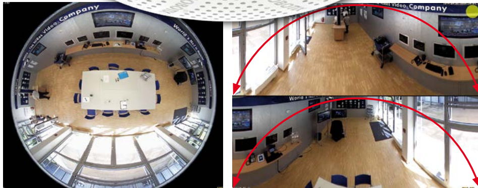
The ceiling-mounted c25 delivers two 180° panorama images of a room.
