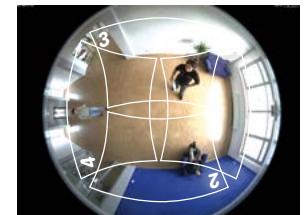
Four virtual PTZ cameras out of a single 360° hemispheric camera
