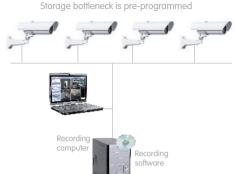
Combining high-resolution video with in-camera-recording means fewer cameras are needed and direct recording to any type of storage device such as, in-camera SD card, Hard Disk or NAS is possible.
