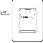
Installation of the light level sensor unit to the C-Bus network requires a two wire connection to the safe extra-low voltage unshielded twisted pair C-Bus network cable. This connection is polarity sensitive, and is clearly marked on the terminal block of the unit. The light level sensor incorporates an LED indicator, which can be configured to aid in identifying the unit during the installation process. This indicator is located on the front of the unit.
