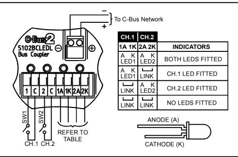
**IMPORTANT** – The LED output connections must be made and maintained orrectly for the unit to operate. **The factory fitted wire link should only be removed if an LED connection is to be made.**
