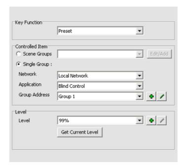
With these settings the relay will remember where it is regardless if controlled by the buttons or sliders.
