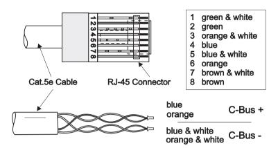
Figure 11. C-Bus network cable connections
