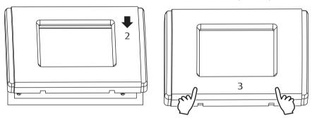
Figure 10. Attaching the fascia (Wall Mounted Touchscreen)
