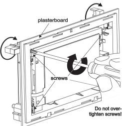
Figure 6. Tighten the screws and the mounting flaps rotate and clamp the wall
