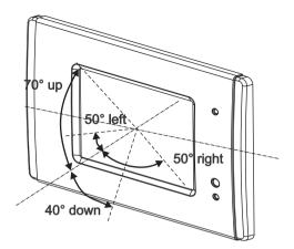
Figure 3. Wall Mounted touchscreen unit's viewing angles
