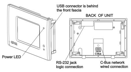
Figure 1. Wall Mount touchscreen connection points
