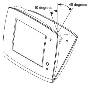
Figure 4. Desktop unit's angle of tilt
