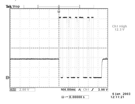
The waveform is sent from the ballast to the DSI unit in a period of roughly 128ms. This is shown in the figure below.
