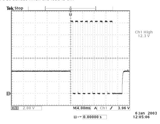
You will notice in the figure directly below, the spacing between the AC voltage changes as the dimming level changes. This is roughly about the 50% mark (visually from the fluro).
