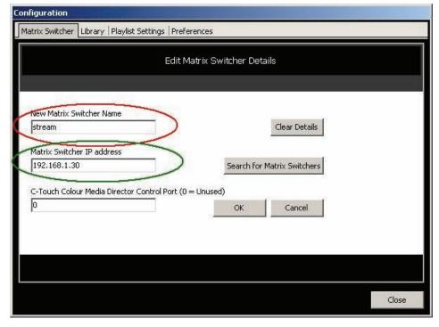
Enter the preferred name for your matrix switcher (suggest something like stream or streaming if you only have a single matrix switcher) in the highlighted red area, followed by the IP Address of the unit in the highlighted green area. If the IP address of the matrix switcher is unknown, click the Search for Matrix Switchers button that will look for available matrix switchers on the network. Clicking OK returns you to the previous screen.
