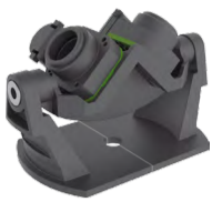
2 image sensors on Pano lens bridge
