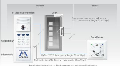
For additional information on the other connection variants and for installing, see the T24 System Manual Part 1 on www.mobotix.com > Support > Manuals
