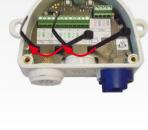
Mount the cover back onto the MX-Input-Box and tighten it using the cover screws (torque 0.4 Nm).
