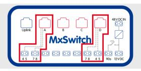
For these two ports, the wire pairs 4/5 and 7/8 have been looped through to the terminals so they can be used for other purposes (see also section *«Example Scenarios»* and the connection examples on page 2).
