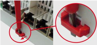
After removing the module, lightly press on the clips; they will jump back into their original position.
