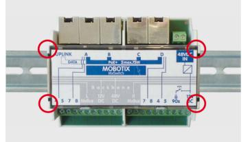
After the clips have clicked into place, you can easily slide the module on the rail until you have positioned it properly.
