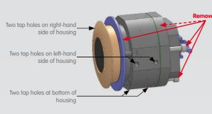
The housing can be installed by affixing suitable screws M4 (4 mm length of thread) in at least two of the six tap holes Remove pressure plate and cylinder head screws.
