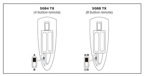
Figure 3 - The Bank selection switch is located behind the back cover
