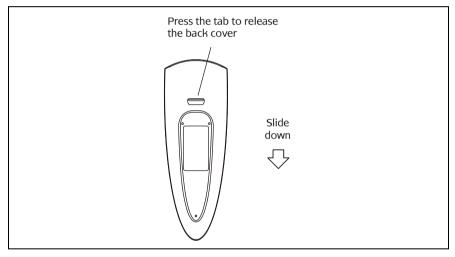
Figure 5 - Removing the back cover to access the battery compartment
