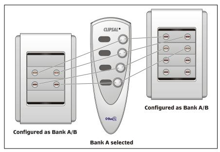
Figure 1 – Neo buttons controlled by a 4 button 5084TX remote
