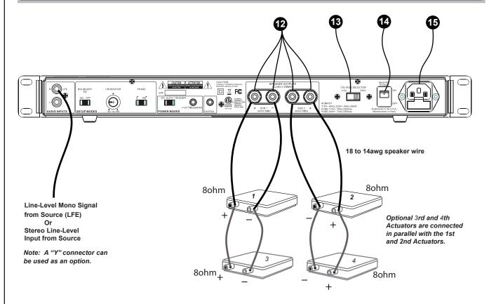
Figure 2: Line-Level and Speaker Level Connections.
