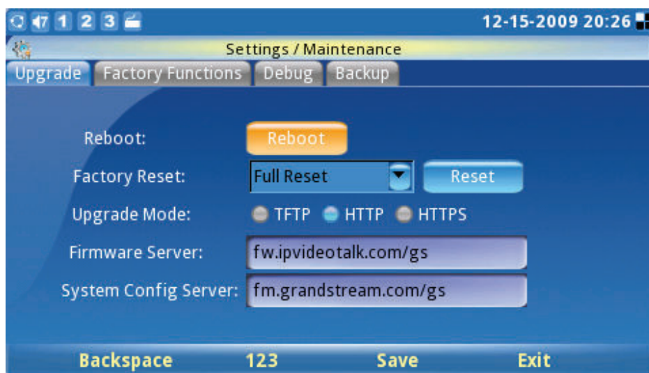
Figure 156: Factory reset the phone using the keypad
