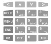
Each time a key is pressed, a short "beep" will be emitted to indicate that the key press was accepted. (The Installer can disable the beeping if necessary)
