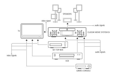
If you prefer, or if your TV does not have sufficient connections, you can connect the audio and video outputs to the CLASSIK Movie System Di. If you have the European version of the CLASSIK Movie System Di you can do this by daisy-chaining your auxiliary components and having one connection to the unit – see diagram below.
