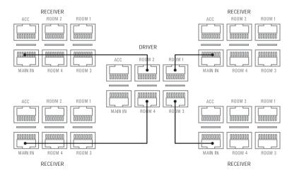
The driver unit feeds a standard stereo audio signal to the receivers, therefore a pair of suitable speakers need to be attached to each receiver in the system.
